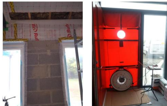
Figure 3: Air Tightness Testing Examples
